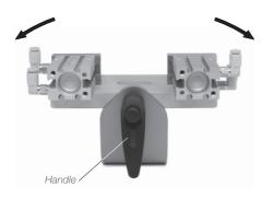
To pivot the CS2R, loosen anf tighten the handle to turning it. The Handle can be aligned vertically again by pressing the Push Button.
